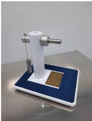
Unscrewing Torque Device
