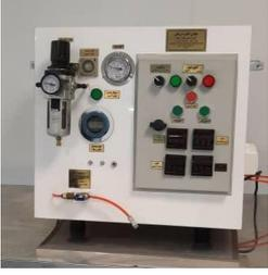
Automated Leakage by Pressure Decay Tester & Sub atmospheric Pressure Air
